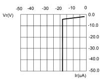
FIG.2 REVERSE CURRENT VS. REVERSE VOLTAGE.
