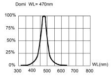
FIG.4 RELATIVE LUMINOUS INTENSITY VS. WAVELENGTH.
